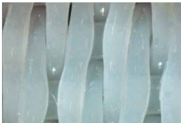
Woven fabric polyamide monofilament
